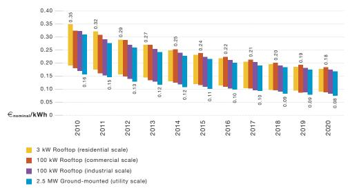
Figure 8 - European PV LCOE range projection 2010-2020 by segment
